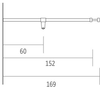
Required pin distance from the installation surface is 167 mm.
