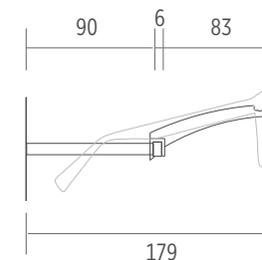
The distance between the top of the frame holder and the back panel is 179 mm.
