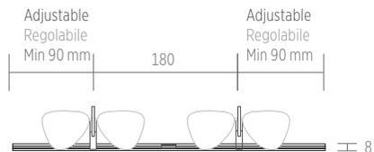
The depth and width of the plate can be adjusted to fit existing units.
