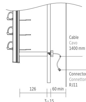
Required distances between the rod and the back panel (3-15 mm thick) is 126 mm. Minimal distance required for the electrical parts (cable RJ11 connector) is 60 mm.
